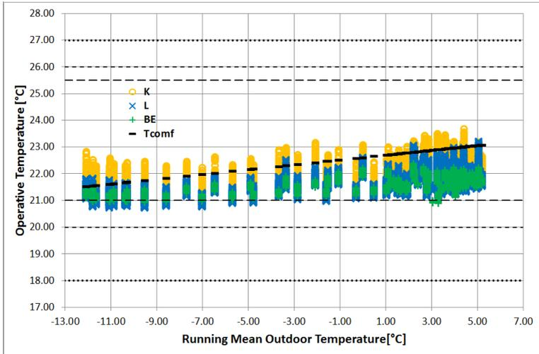
Fig. 4. The operative temperature of areas **L**, **K** and **BE** together with the calculated value of comfort temperature based on  $T_{rm}$ , as a function of  $T_{rm}$  using natural ventilation and convection heating. The broken lines represent ranges of  $T_{op}$  for each category: long line – I (high level of expectations), short line – II (standard level of expectations), dot – III (acceptable level of expectations).
