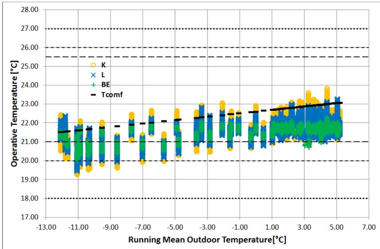
Fig. 5. The operative temperature of areas **L**, **K** and **BE** together with the calculated value of comfort temperature based on  $T_{rm}$ , as a function of  $T_{rm}$  using natural ventilation and underfloor heating. The broken lines represent ranges of  $T_{op}$  for each category: long line – I (high level of expectations), short line – II (standard level of expectations), dot – III (acceptable level of expectations).
