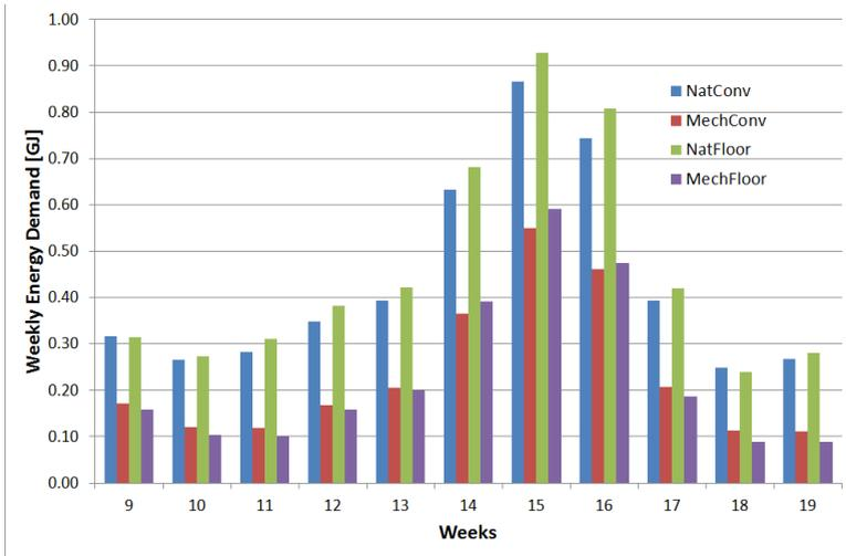
Fig. 8. Comparison of weekly energy demand for the building using different variants.
