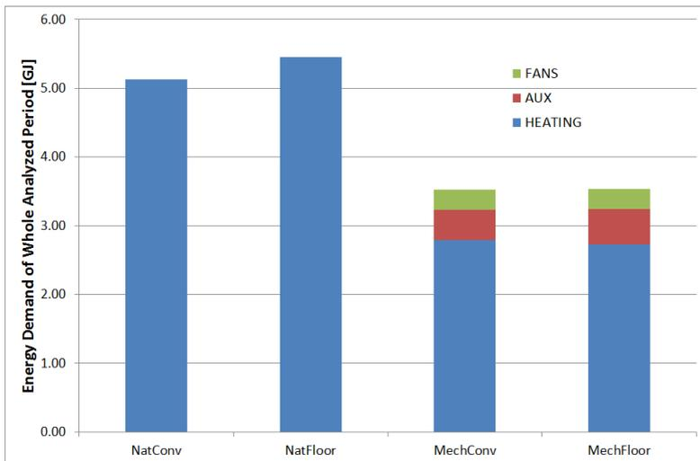
Fig. 9. The share of heating and energy for appliances in the total energy demand of the apartment in the analyzed period.
