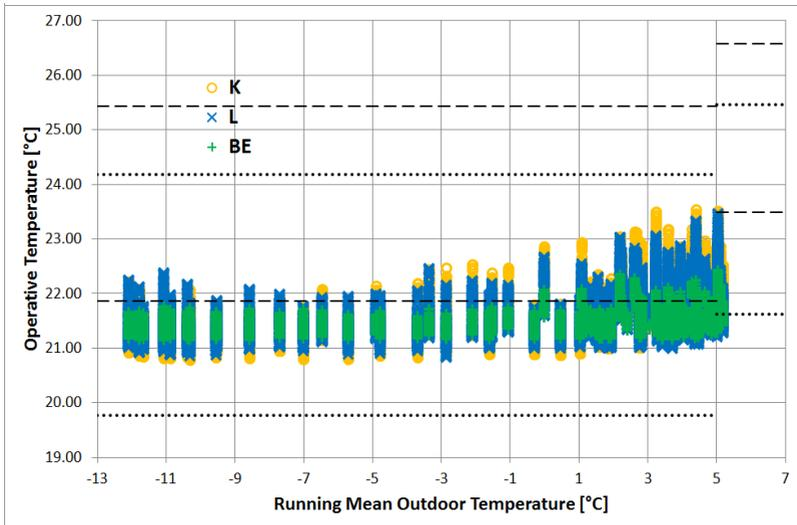
Fig. 7. Operative temperature of areas **L**, **K** and **BE** as a function of running mean outdoor temperature in terms of mechanical ventilation and underfloor heating. The broken and dotted line represent the  $T_{op}$  values ensuring that PMV is between -0.5 a 0.5 (category II in [9]) for physical activity of 1 and 1.2 met respectively.
