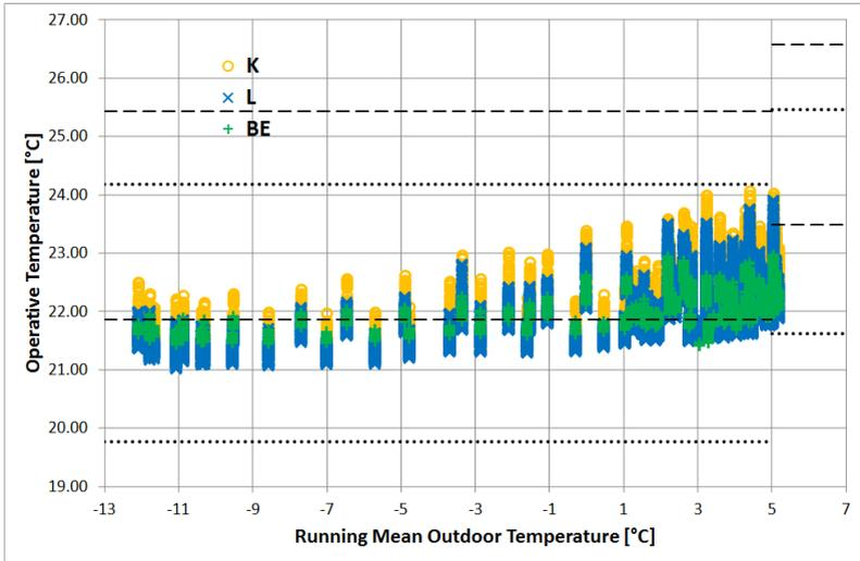
Fig. 6. Operative temperature of areas **L**, **K** and **BE** as a function of running mean outdoor temperature in terms of mechanical ventilation and convection heating. The broken and dotted line represent the  $T_{op}$  values ensuring that PMV is between -0.5 a 0.5 (category II in [9]) for physical activity of 1 and 1.2 met respectively.
